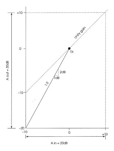
been expanded since minimum output level is now 10dB less than minimum input level. In other words, the dynamic range has been expanded downward.
